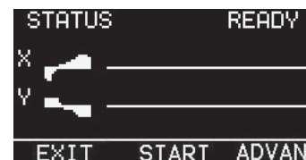
Figure 12a. Once calibration is complete, the STATUS READY screen appears with a tracking error graph.
