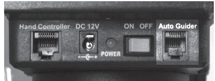
Figure 3a. The Solitaire works with any mount equipped with an ST-4 compatible autoguider port, shown here on the Sirius EQ-G mount.
