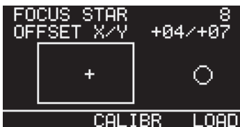
Figure 9. This screen displays the guide star focus quality and its relative location on the camera’s detector.
