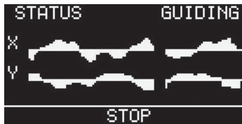
Figure 12b. Select START to begin autoguiding. The tracking error graph will display during autoguiding.
